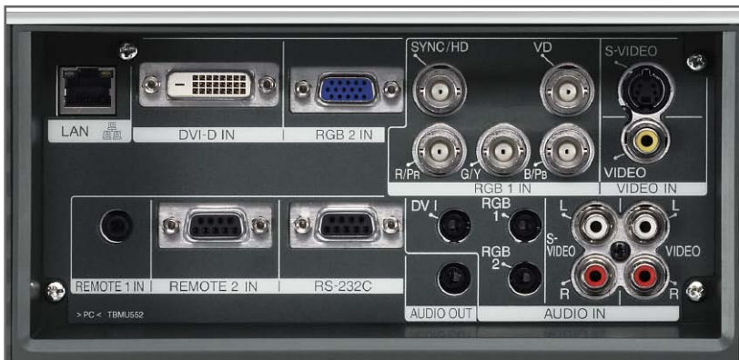
Terminals include an HDCP-compliant DVI-D input connector
